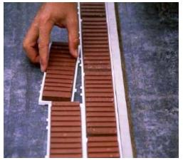
Figure 2: Snapping the bricks together
