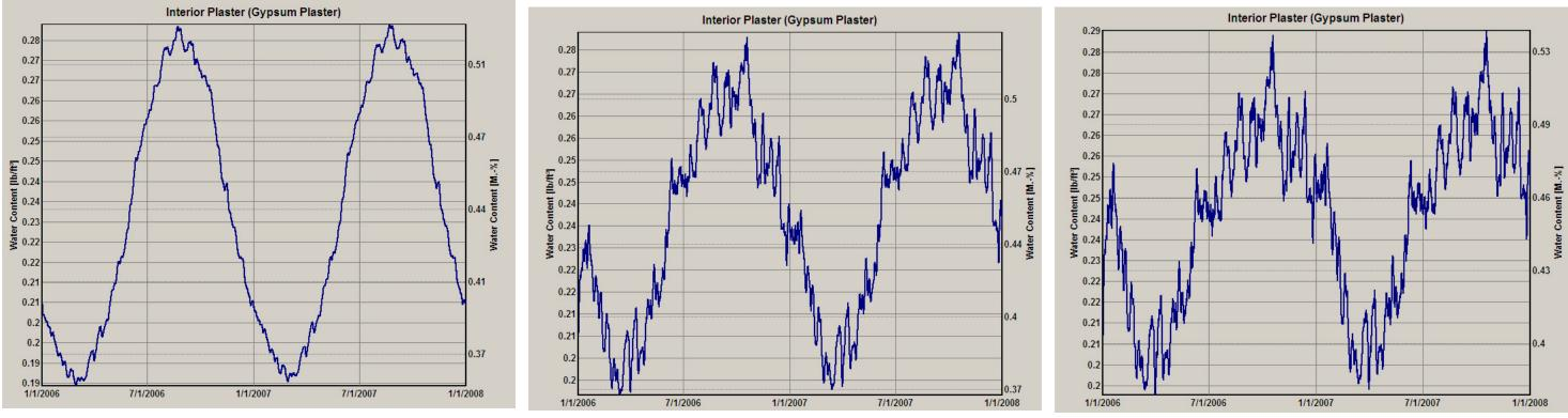
Figure 10: Water content of the interior surface during a 2 year period for panel with insulation, panel without insulation with airspace, panel without insulation without airspace
