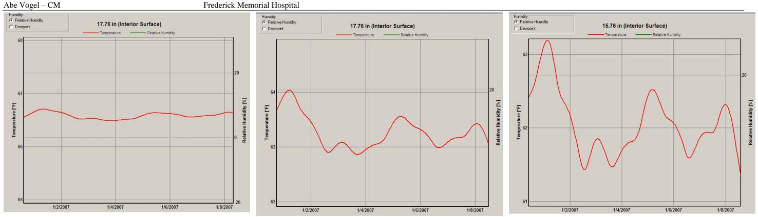
Figure 9: Temperature on interior wall during 1 week period in January for panel with insulation, panel without insulation with airspace, panel without insulation without airspace
