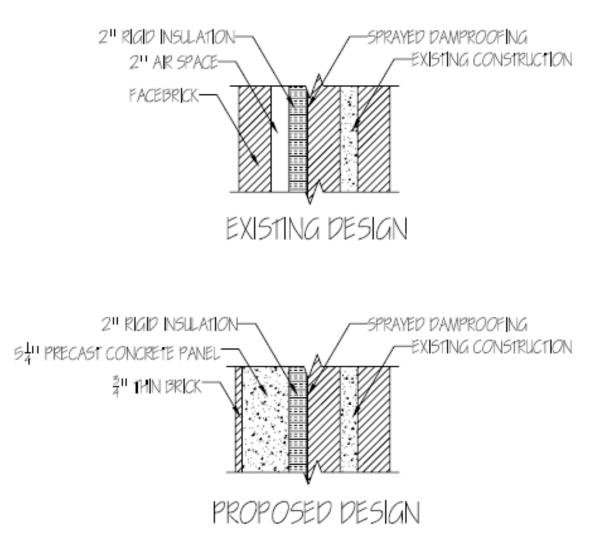
Figure 3: Proposed v. Existing Cross-Sections
