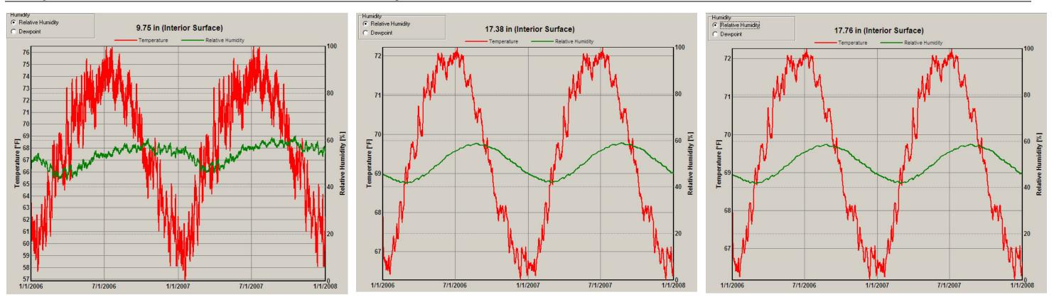
Figure 4: Temperature on interior wall during 2 year period for old façade, existing veneer design, and proposed panel design
