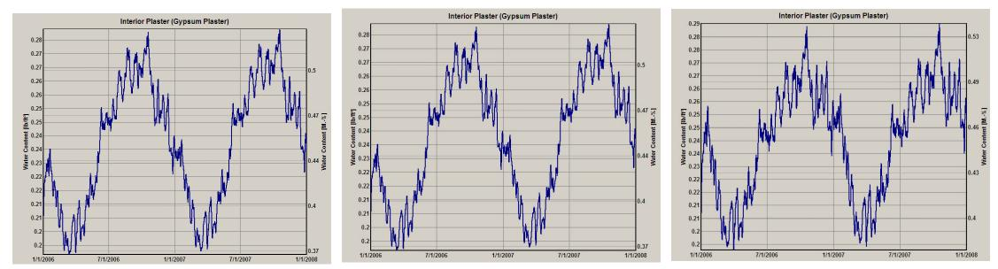
Figure 8: Water content of the interior surface during a 2 year period for panel with airspace with damproofing, panel without airspace without damproofing, panel without airspace without damproofing.
