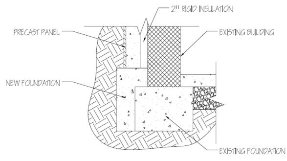
Figure 12: Schematic Design of New Foundation
