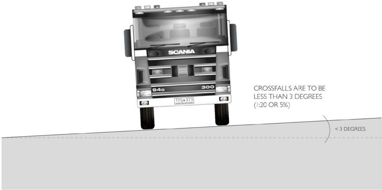
Figure 1 Cross fall angles
