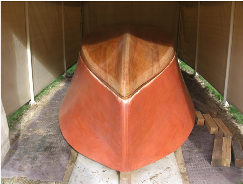
“The bottom has been fiberglassed and the sides of the hull & transom have been stained.”
