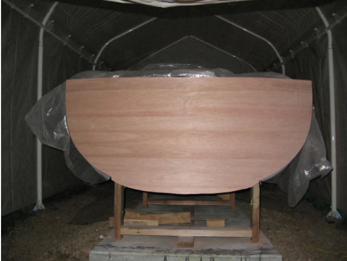
“Transom mahogany sanded and ready for paint and stain.”
