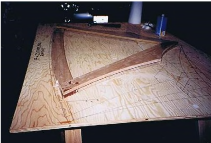
"Constructing frames on the plywood layout table."
