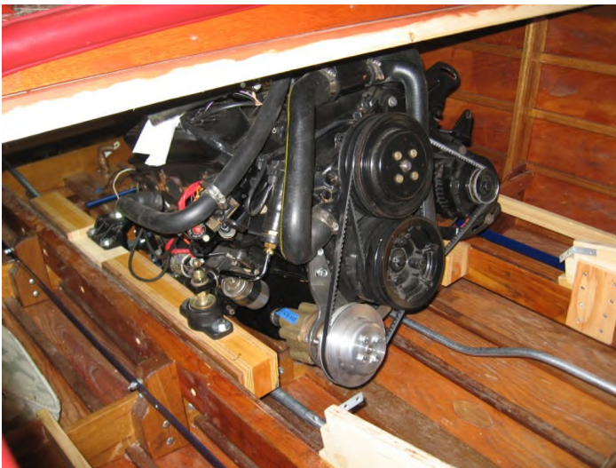
“Engine view with rear seat removed. The rear seat back can be removed to expose opening in rear seat back support that allows access to the front of the engine for maintenance.”
