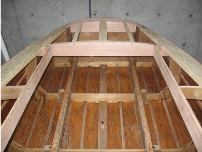
“Deck framing started.”
