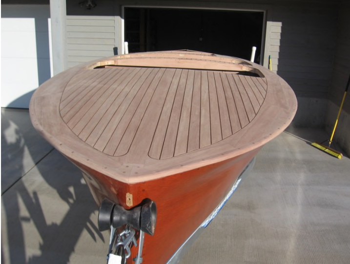
“Decking installed and ready to be finished.”
