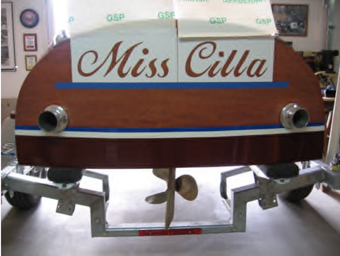
“Stencil in place on transom ready to place sizing and gold leaf.”
