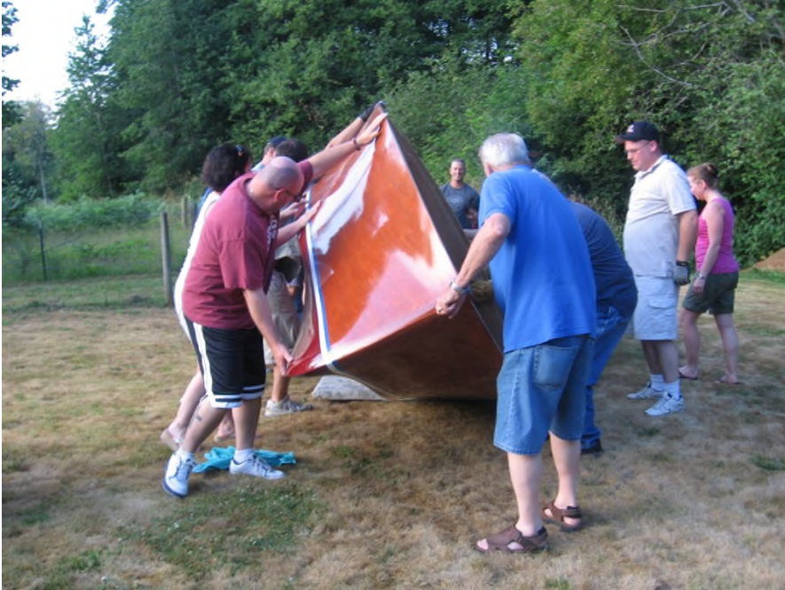
“Rolling the hull over on a mattress pad.”
