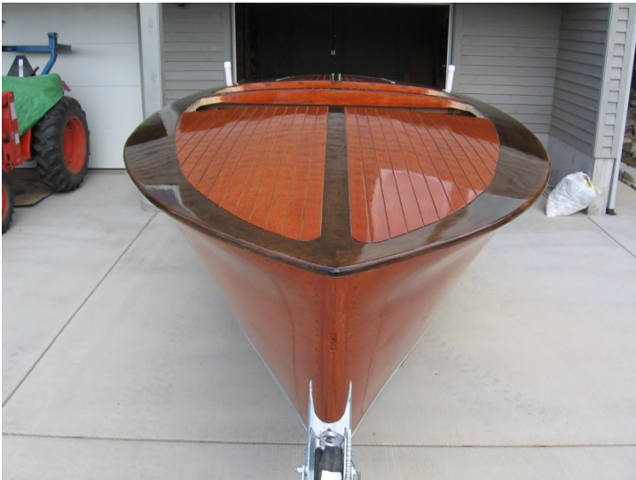
“Deck has been finished, ready for white joint deck caulking and installation of hardware.”
