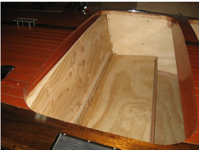
“Interior rear seating, side panels and flooring being installed.”
