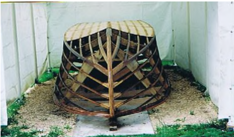
“The frame is complete, faired, and some sheathing is being installed.”
