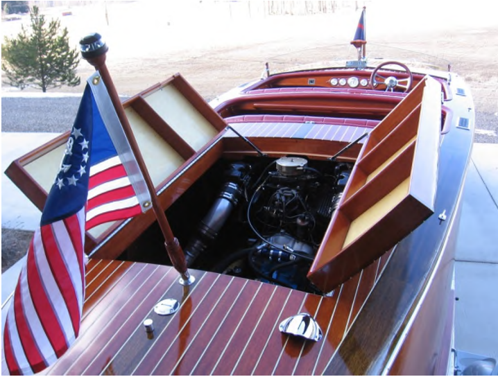
“Engine installation complete with motor hatch doors reinstalled.”
