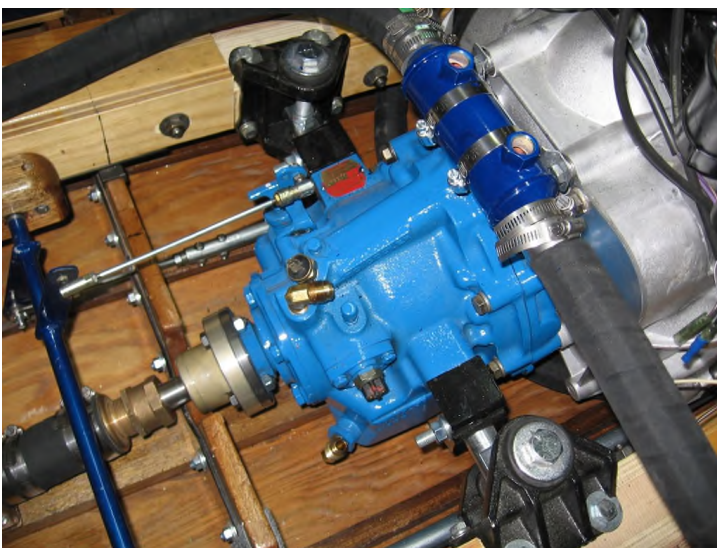
“Transmission linkage and transmission oil cooler in place.”
