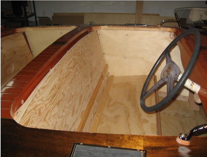
“Interior front seating, side panels and flooring being installed. Beginning installation of Steering box. The steering box is from a 1951 GMC Pickup. The steering column will be shortened and a new steering wheel will be added.”
