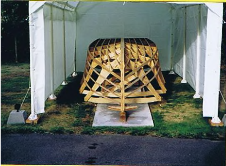
“The frame a little more complete with the canvas carport for weather protection.”
