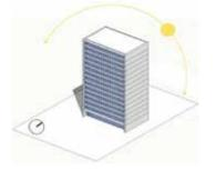
[Figure 14] Minimise solar heat gain by reducing openings on the East or West façade.
