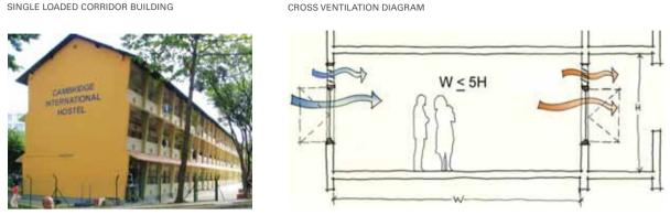
[Figure 6] Design of natural ventilated spaces.
