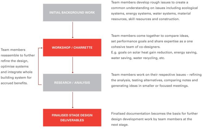
[Figure 2] An integrated green building design approach.
