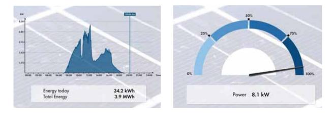
[Figure 19] Examples of live performance monitoring displays from an SMA inverter. Source: Phoenix Solar
