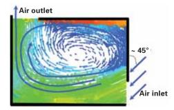
[Figure 8] Wind enters inlet at 45° and circulates within room before exiting from outlet.
