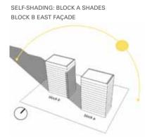
[Figure 17] Use of massing to provide shading for multiple blocks.
