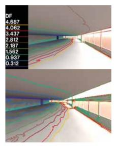
[Figure 7] Daylight simulation showing an office space without light shelves (top) compared to an office space with light shelves (bottom). Daylight distribution is better with light shelves, with less glare at the perimeter zone next to the windows.
