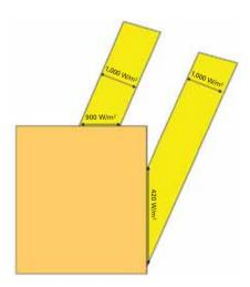
[Figure 9] Equatorial sun shines more intensely on the roof than the walls.
