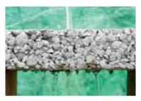
Source: gaia engineering [Figure 11] Examples of porous concrete.
