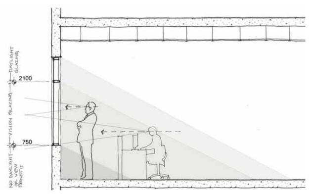
[Figure 4] Effective height of daylight glazing.
