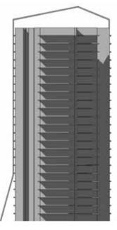
[Figure 19] Rotation of south facing façade to provide more shade at the hottest time of the day.
