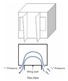
[Figure 17] Wing walls improve ventilation into a space where openings can be made only on one side of the space.
