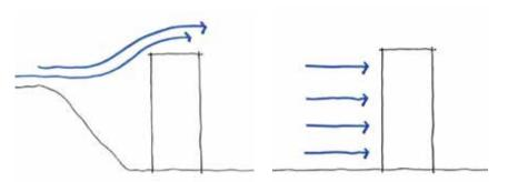
[Figure 9] Location of building resulting in different wind conditions.
