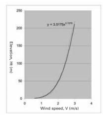
[Figure 9] Wind profile used for boundary input.
