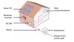
[Figure 7] Grid-tied system configuration.
