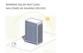
[Figure 16] Minimise solar heat gain by adding balconies as shading devices.
