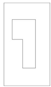
[Figure 10] Same floor area with varying building perimeters – greater perimeter constitutes greater material use and cost for building envelope.
