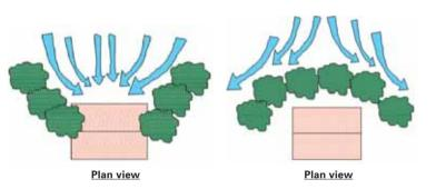
[Figure 11] Vegetation can divert wind to flow (left) towards or (right) away from a building.
