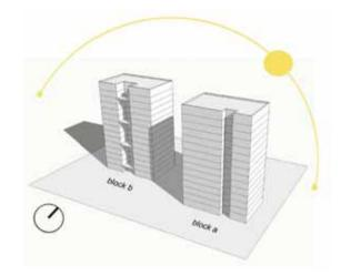
[Figure 18] Use of building mass or overhang to produce shadow / shade.
