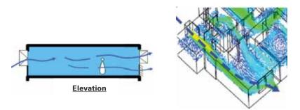
[Figure 7] Wind driven cross ventilation.
