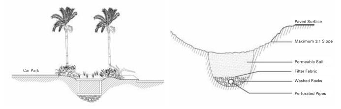
[Figure 6] Section showing a bioswale.
