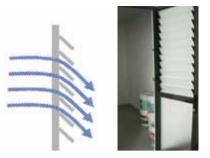
[Figure 20] Section view of louvred door / window. It has the effect of deflecting airflow downwards and reducing the airflow into the space depending on its percentage of perforation.
