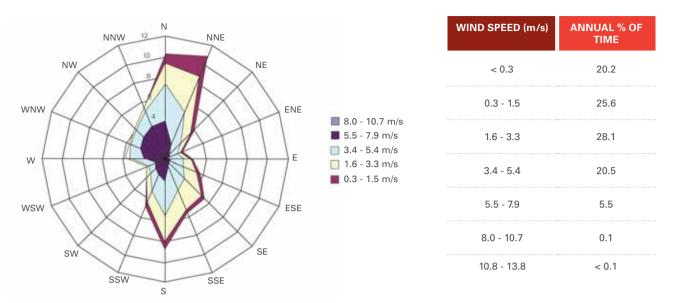
[Figure 3] Wind data from Meteorological Service Singapore – Changi Station 1975 - 2006.
