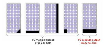
[Figure 13] Examples of partial shading on a 36-cell module.
