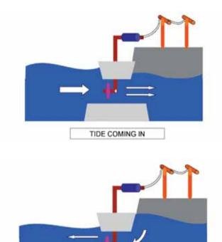
[Figure 6] Illustration of tidal energy generation during high tide and low tide.
