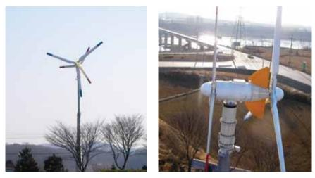
[Figure 2] Examples of Horizontal-axis wind turbines (HAWTs). 6 bladed wind turbine generator installed beside conventional 3 blade wind generator – near Bi-young Bridge at Kyunggi-Do South Korea.
