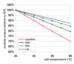
[Figure 12] The effects of negative temperature coefficient on module performance.
