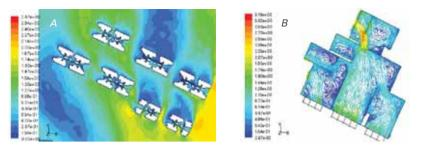
[Figure 23] Air velocity contour plots at estate level (left) and vector plots at unit level (right) conducted for HDB's demo eco-precinct: Treelodge @ Punggol. Source: HDB
