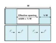
[Figure 19] The effective opening size of a casement window unit depends on the manner of sliding its leaves.
