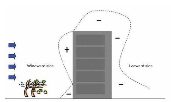
[Figure 4] Positive and negative pressure on windward and leeward side respectively.
