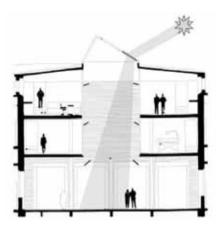
[Figure 6] Daylighting strategy for internal circulation space.
