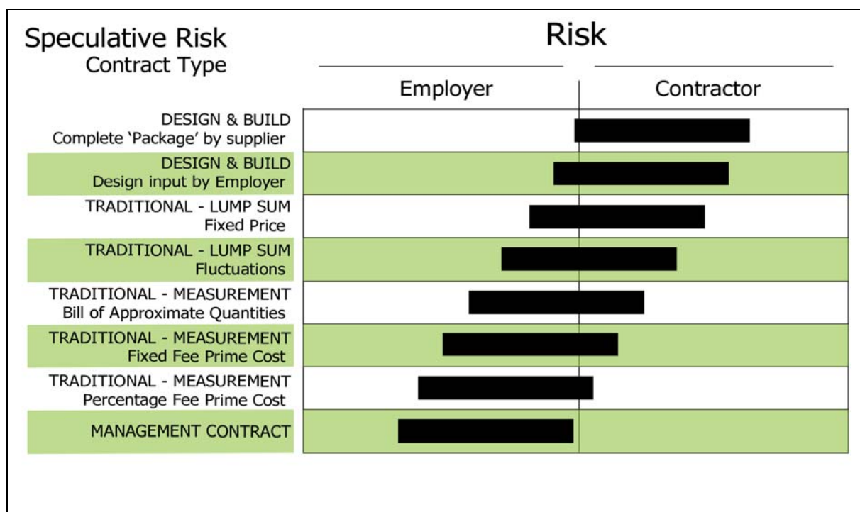
Figure 1 Risk apportionment between client and contractor
