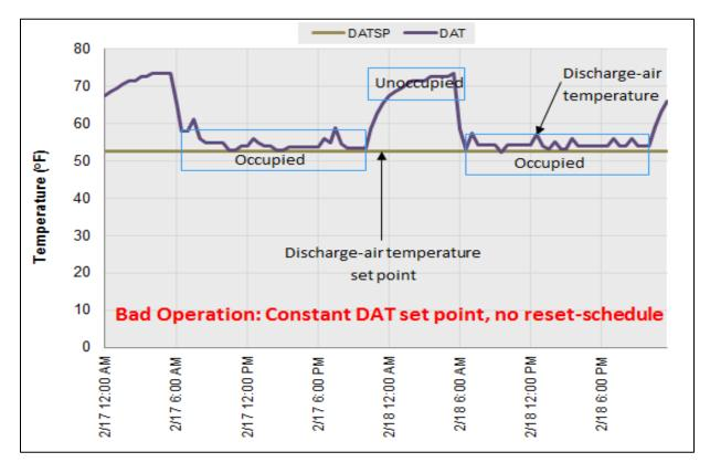
Figure 1: No discharge-air reset-schedule in place.
