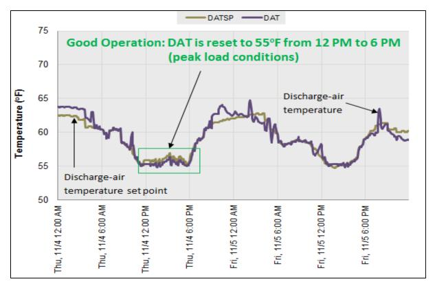
Figure 2: Air-handler with good discharge-air reset-schedule.
