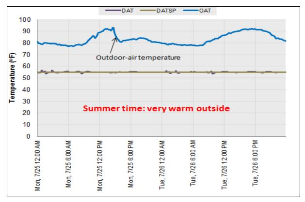
Figure 5: Discharge-air temperature and set point for an air handler.
