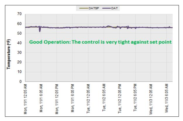
Figure 8: Discharge-air temperature very steady against the set point.
