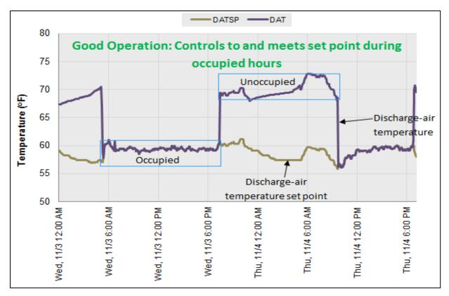
Figure 4: Discharge-air temperature controls to set point very well.
