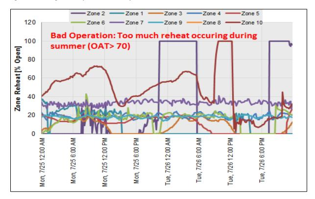
Figure 6: Reheat valve signals vs. time for zones served by AHU in Figure 5.
