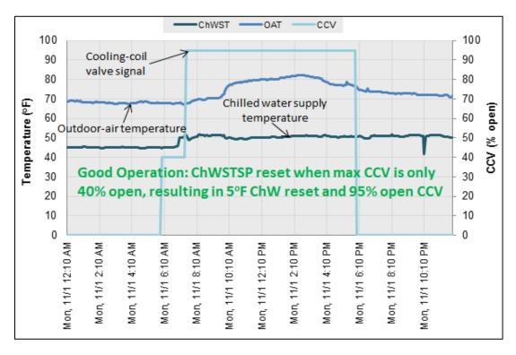
Figure 4: Example of good operation, where the chilled water supply temperature set point is reset by 5°F, and the cooling-coil-valve signal responds by opening 95%.
