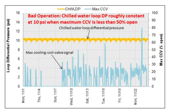
Figure 7: Example of bad operation, where the loop differential pressure is not reset when the maximum cooling-coil-valve signal is always less than 50% open.
