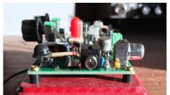
Mount the circuit board to the breadboard with four 1/2 inch brass wood screws and black 3/8th inch plastic spacers. You should have starter holes on the breadboard (Breadboard step 4.) You may need to loosen or remove the key to get the front right screw in.
