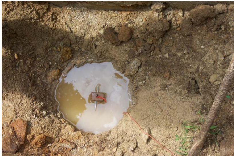
Figure 2- Soil Percolation Test
