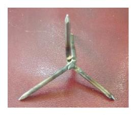
angle. The final step was to weld the two nails together, to form the final caltrop.
