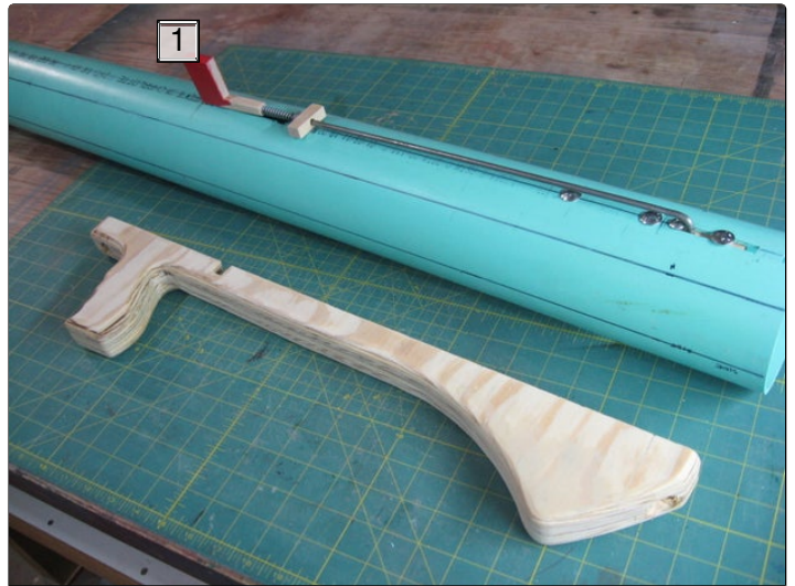
1. This entire piece is attached first, and then the handle is bolted in place over it. This set-up is nice because everything can quickly be broken down if need for adjustments or repairs.
