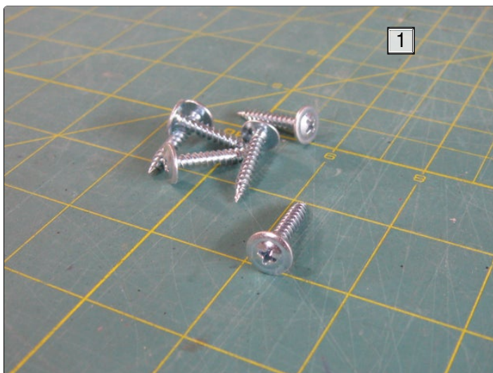
1. Metal-to-metal pancake head screws. They work well in this project because of the low profile of the screw head.
