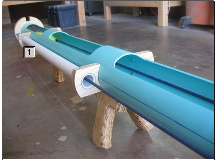
1. Rear handle section, which houses the trigger mechanism.
