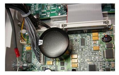
**3.** Disconnect the cable connectors on the power supply board.
