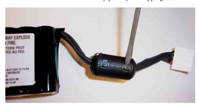
Figure 4-1: Example of ferrite removal for the Burdick 8300
