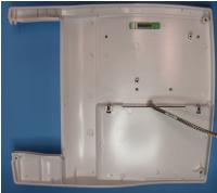
ECG device Top Cover Assembly (with Video Display)
