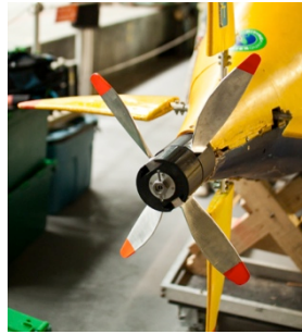
Figure 14. Single-axis contra-rotating propellers for the 2013 design (pictured on Minerva ).
