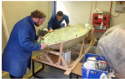
Figure 11. Vacuum bagging the wet layup hull.
