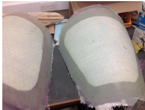
Figure 13. Honeycomb core conforms to complex curvatures in the hull.
