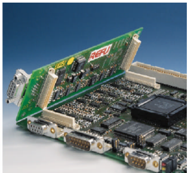
Subminiature connectors in 1.27 mm grid Termination: SMT, press-fit or solder pin and IDC for ribbon cable Board to board heights: 8.0, 9.4, 10.8 or 12.2 mm
