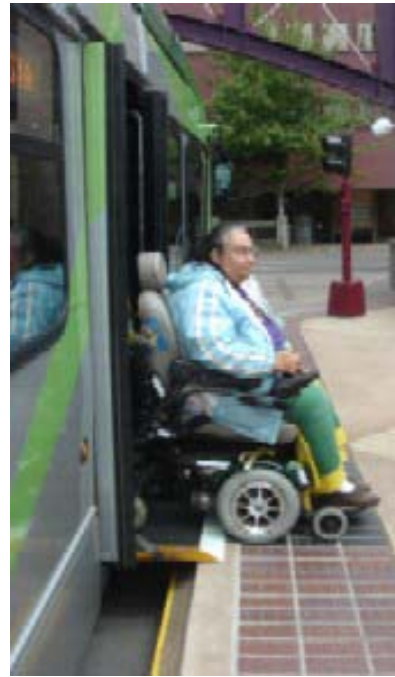
Near-level boarding on the EmX.
