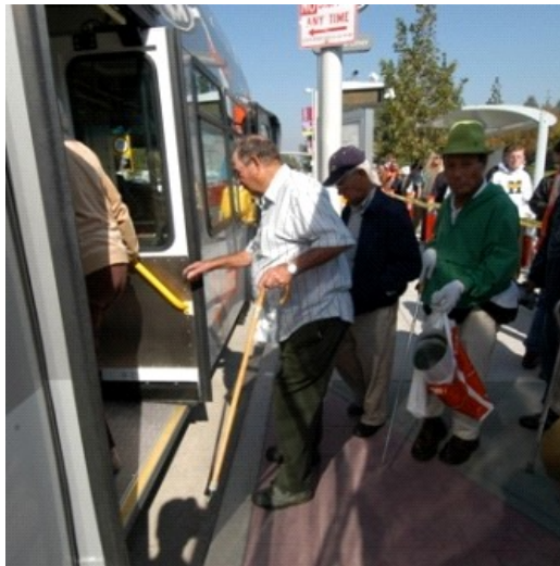
A 6-inch step for passengers on the Orange Line.
