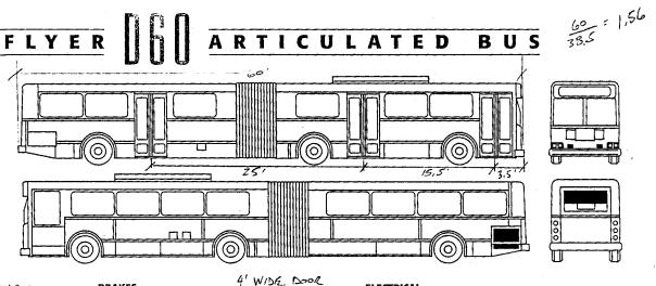
· Reinforced fiberglass exterior roof, front & rear and aluminum side panels for maximum corrosion resistance and reduced maintenance.
