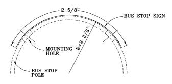
SIGN TO BE CURVED TO FIT 2 3/8" OUTSIDE DIAMETER BUS STOP POLE.
