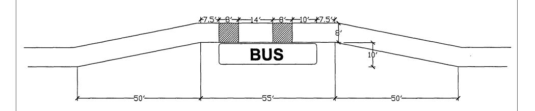
SHADED AREAS SHOWN ON SIDEWALK ADJACENT TO THE BUS STOP SHALL BE CLEAR OF ANY PHYSICAL OBSTRUCTIONS.
