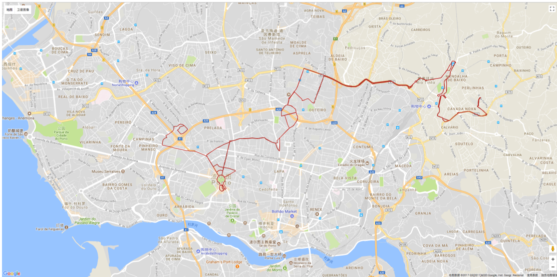
(b) After snapping, the polyline is tighter and the route is clearer.
