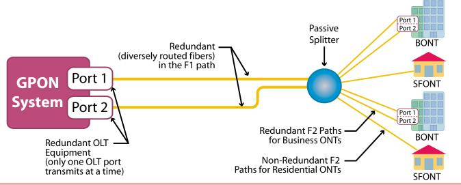
Figure 4: Type B Protection Scheme
