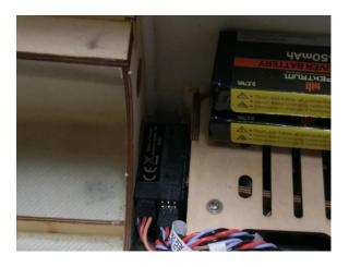
This example on a BVM plane used a regular Spektrum 9030 Rx and a X-plus expander. You can find the Rx channel mapping under Connecting Rx wires later in this manual.
