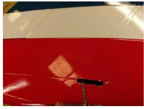
☐ Use a 1/16" Carbide Cutter to add some glue holes as shown.
