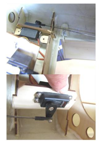
☐ Lift the servo mount up as shown. The wire linkage should slide out of the slot in the #3 bulkhead. The servo could be changed with this access.
