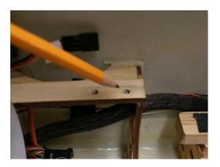
We recommend using some Qt poxy to hold the blind nuts in place. BVM # PA-SR-0042
