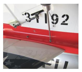
**NOTE**: The elevator neutral position is located as shown.
