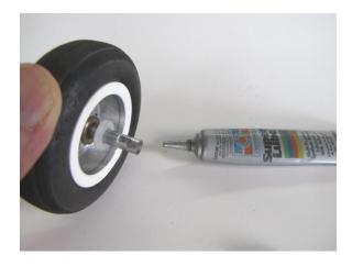
Reassemble the wheel, brake, and axle. Use a small drop of thread locker on the set screw. Check for free spin of wheel and brake application.
