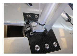
Use a 1.5mm hex wrench to loosen the set screw that retains the axle. Check to see if there is a flat spot ground in the axle. If not, use a dremel cutting disc to make one as shown. A matching cutter mark on the end of the axle helps to properly orient it.
