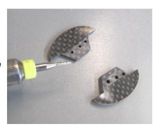
☐ Use ZAP-RT or similar rubberized glue to attach the Skidz as shown. Wipe away excess before it cures.
