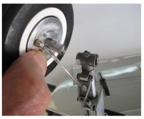
□ Apply Parker Super "O"Lube to the brake "O"Ring and on wheel inner drum.BVM #5779
