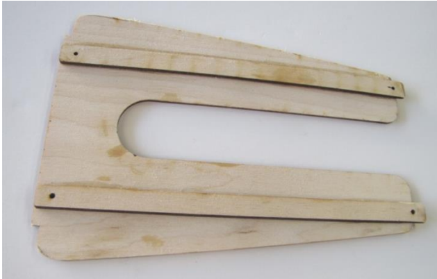
View of bottom side of battery tray
