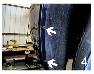
**4.** Forward of front tires are two screws to remove from wheel well edge with the Phillips screw driver, both sides.
