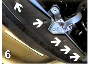
6. Remove five christmas tree push pins from lower edge of fascia next to motor mount. Pull fascia forward, unplug electrical connection to fog lights (available with some models) and set aside.
