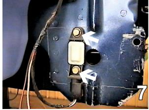
7. Using the 10MM socket, remove two metric bolts from the air bag sensor, both sides and tie up out the way.
