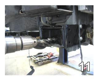
11. Using the 17/32" drill bit, drill the hole in the front of the baseplate using the baseplate as a template. Do this to both sides.
