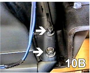
10. Insert the 3/8 x 1 1/2" hex bolts into baseplate and drilled holes, tighten 3/8" lock washer and hex nut on the back side of webbing with the 9/16" socket, both sides. Be sure and use Loctite on all bolts before tightening. Tighten all bolts according to Torque Chart in the General Instruction Sheet.
