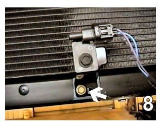
Remove one metric bolt from the temperature sensor using the 10MM socket and set out of the way.
