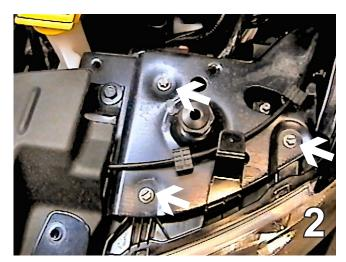
2. Remove three metric bolts from headlight assembly with the 8MM socket, pull forward, unplug electrical and set aside, both sides.
