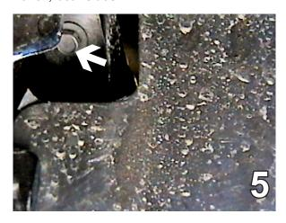
**5.** Remove the one metric bolt just forward of the front tire, on fascia's corner, using the 8MM socket, both sides.
