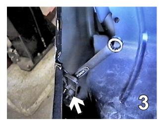
Just behind headlight assembly is one metric bolt to remove with the 8MM socket or wrench, both sides.
