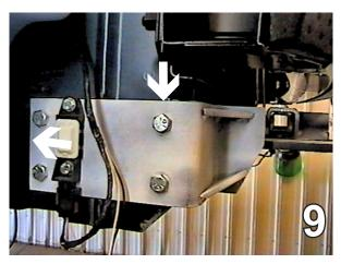
9. Align back and top edge of baseplate even with the webbing on the lower frame and clamp in place. Obround holes on baseplate end need to be aligned with existing air bag sensor hole locations. Be sure baseplate is level. Drill the four holes in the webbing with the 13/32" drill bit, both sides.
