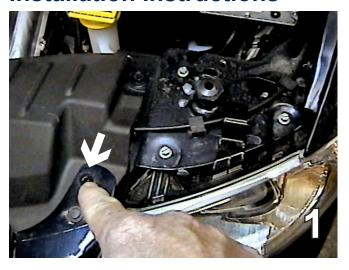
1. Remove one metric bolt just between headlight assemblies on top edge of fascia, with the 10MM socket, both sides.
