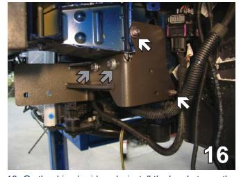
16. On the driver's side only, install the bracket over the top of the studs (white arrows). Tighten with a 3/8" flat washer for the top stud, 3/8" lock washers and 8MM hex nuts. On the front (gray arrows), attach 3/8" flat washers, 3/8" lock washers and 8MM bolts to the existing nuts.
