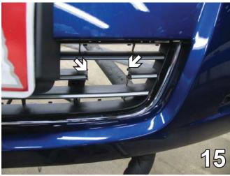
15. Using the hack saw blade, cut out the fascia middle horizontal rib to the outside of the sensor. Remove the whole piece to open the area up for baseplate installation. Do this on both sides of the vehicle.
