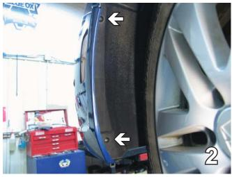
2. Using a 20 Torx, remove two screws from just forward of the front tire on the edge of the wheel well cover. Set screws aside to be reinstalled later. Do this to both sides of the vehicle.
