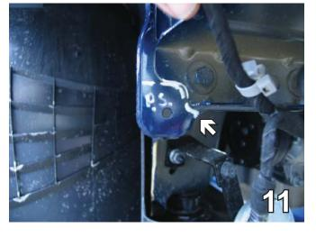
11. On the passenger side, cut around the ridge to the top then straight out.
