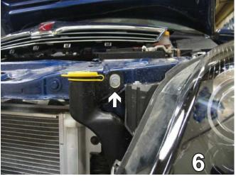
Using the 10MM socket, remove the top metric bolt from the washer reservoir. Set the bolt aside to be reinstalled later.
