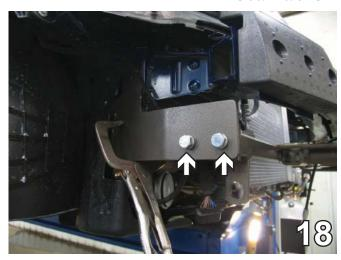
18. Loosely bolt the baseplate cross member piece to the end plates with 1/2" x 1 1/4" hex bolts and 1/2" lock washers. Be sure it is level with the vehicle and clamp to the passenger's side.
