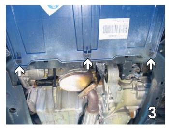
Remove three push pins from underneath on the bottom edge of the belly pan. Set the push pins aside to be reinstalled later.
