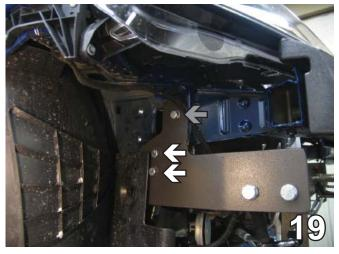
19. On the passenger side, using the baseplate as a template, drill all three holes with the 13/32" drill bit. Insert into the bottom two holes (white arrows) 3/8" x 1 1/4" hex bolts with Loctite Red, tighten with 3/8" lock washers and 3/8" hex nuts. Insert a 2" hex bolt with 3/8" lock washer using Loctite Red into the top hole (gray arrow) and tighten with 1" nut plate. Tighten the baseplate to the end plates.
