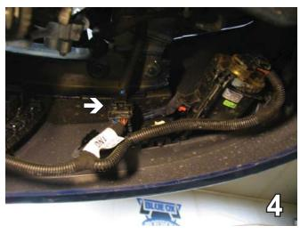
4. On the passenger side only, up in behind the front tire, unplug the master connector.
