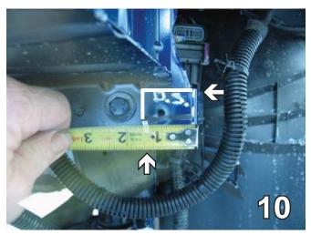
10. On the driver's side, cut off the tab then over 1 1/2" and straight down.
