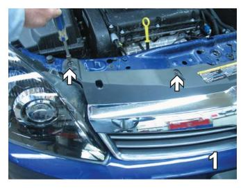
1. Using a 25 Torx, remove three metric bolts from the top side of the fascia. Set the bolts aside to be reinstalled later.
