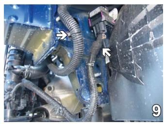
After the washer reservoir is removed, unclamp the two hoses and pull up out of way. Do this on both sides.
