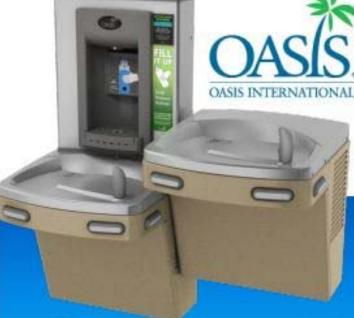
Model: PGF8EBFSL - filter monitor, bottle counter, powder coated finish, galvanized panels and frame, silver ion infused components, programmable lock out, mechanical activation, one-piece molded antimicrobial bubblers, antimicrobial copper push pads, external stream adjustment, high efficiency cooling, adjustable thermostat, stainless tops, universal hi-low install, ADA compliant
