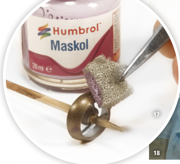
17 With a sponge we apply some Maskol to the front parts of the cowlings as well.
