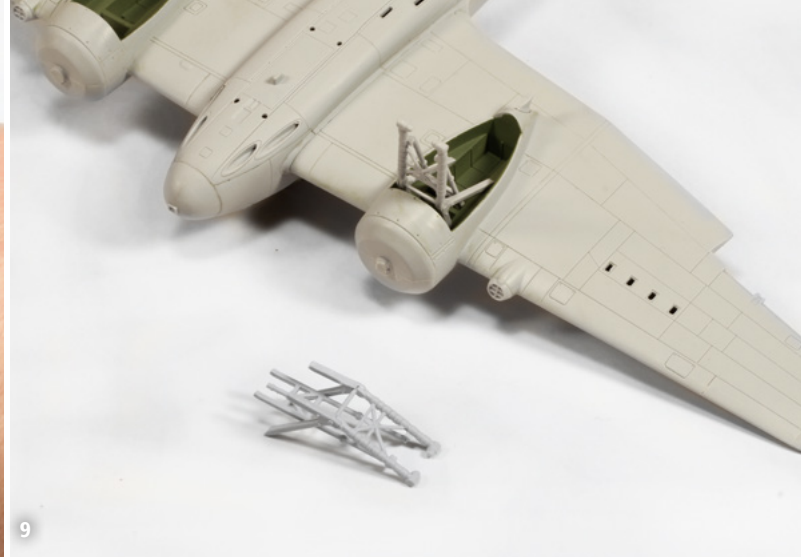
9 The landing gear is assembled and test fitted. This will be left separate for easier painting and weathering.
