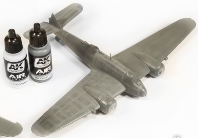
13 And by adding first some white to the base color here also the panelines are sprayed in a lighter tone.
