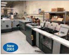
HEIDELBERG SADDLE STITCHER # ST100, 6-PKT COVER FEEDER, SCORING 3-KNIFE TRIMMER, STITCHING HEADS, DELIVERY CONVEYOR
