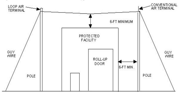
Figure A4.1. Air Terminals on Masts (Typical).
