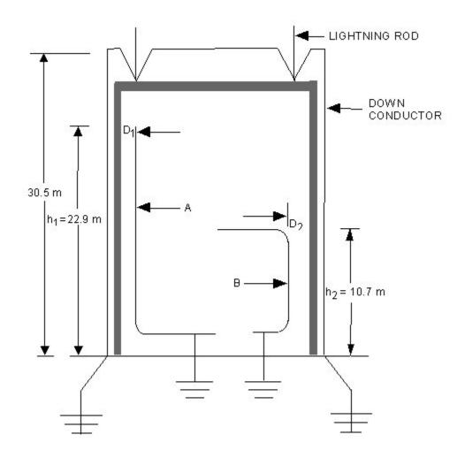
Figure A3.2. Typical Bonding Conditions in Structures Greater Than 12.2 Meters (40 Feet).
