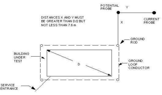
A6.2. Resistance Test for Above-Ground Petroleum (POL) Tanks. The method described in paragraph A6.1 is appropriate for medium to small grounding systems. Figure A6.2 illustrates how to measure resistance to earth of larger, more complex systems such as a large POL tank or a substation. In areas where the soil resistivity is relatively high, a higher voltage supply may be necessary. Local cathodic protection technicians can usually furnish the material for the test.
