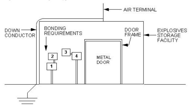
Figure A3.4. Bonding for Typical Air Force Structure.
