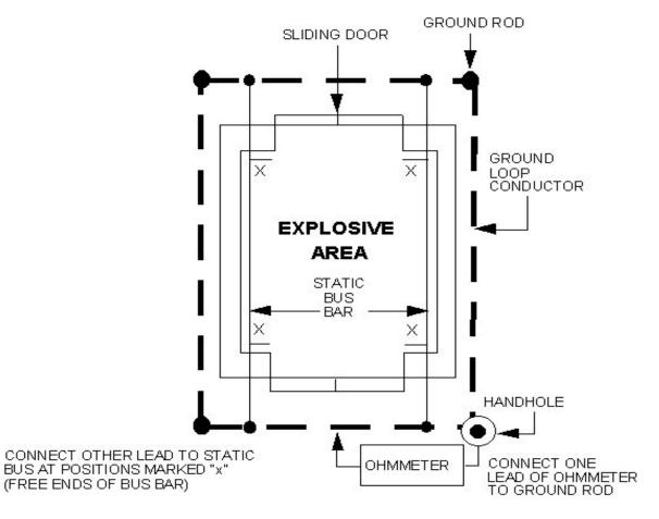
Figure A6.5. Testing Static Bus Bars in Typical Explosives Area.
