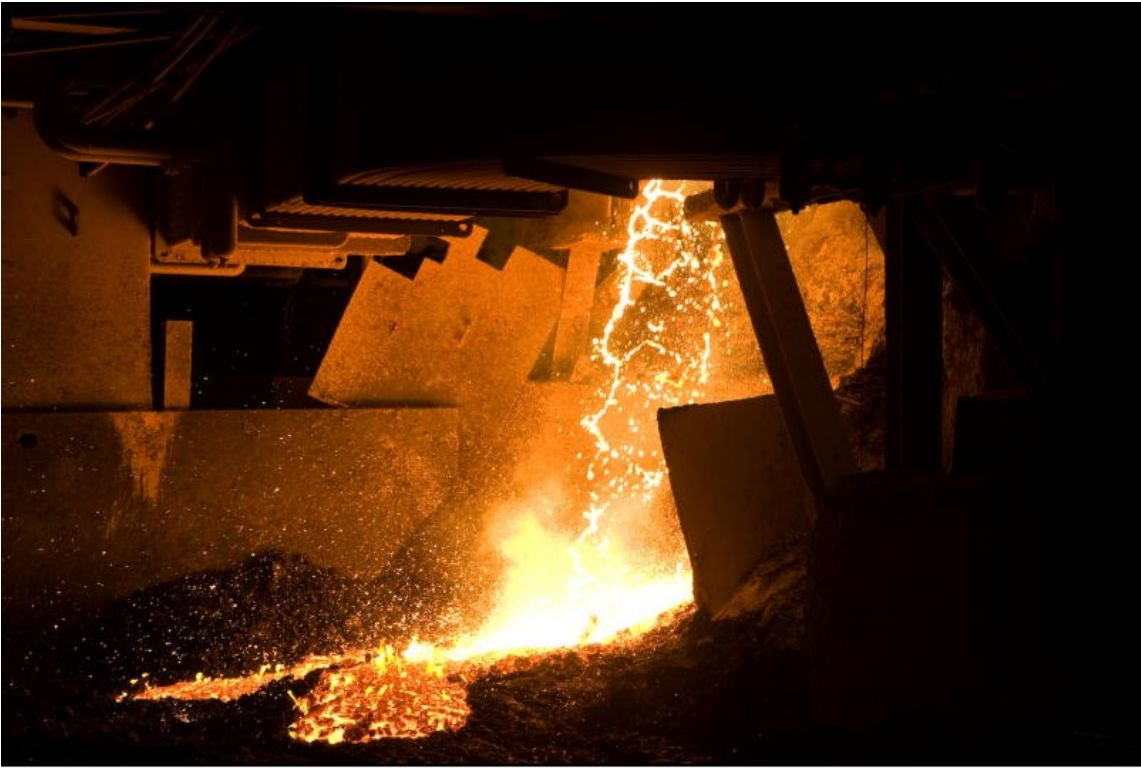
During the steel recycling process, scrap metal is heated in an electric arc furnace (EAF) which requires large amounts of energy that vary significantly depending on the amount of scrap placed in the furnace.
