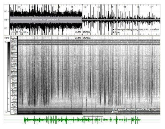
In the picture above is a signal received in my garden with the E202 and 75 cm stylus, without and with receiver connected to ground. Left part without ground connection and Right part with it on. The ground connection reduces the hum noise by 20 dB. Signal processed with Sonic Visualizer software.
