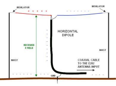
The figure above shows how a horizontal dipole behaves at VLF frequencies. The receiver is not differential but referred to ground, so the received component will always be the vertical one, even with the antenna placed horizontally. This is because the antenna is much shorter than the signal wavelength and therefore does not behave as an antenna but as a field probe. It detects the vertical voltage between two points: the ground and the antenna.
