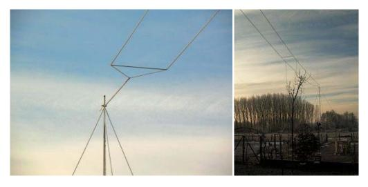
Electrically the Marconi antenna is nothing more than a vertical antenna with a tip that splits and goes horizontally, making a hat. This configuration gives great performance on low frequencies, and for this reason it is also widely used by the military to transmit signals in the VLF band.
