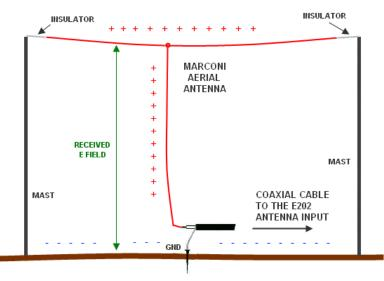
The dimensions are not critical because the antenna is not resonant: 3 meters vertical and 6 meters horizontal are sufficient to provide a large increase in efficiency compared to a 75 cm stylus; especially in the reception of frequencies below 100 Hz.
