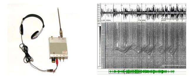
It can be assembled as a compact, lightweight and extremely sensitive receiver. It functions well in the field thanks to an internal battery with autonomy of 40 hours. It will also function as a base station receiver using external power in a permanent monitoring observatory.
