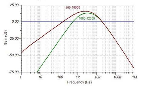
In the graph the frequency response of the receiver with a whip antenna: with (brown curve) and without high pass filter jumper (green curve).
