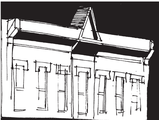
A simplified interpretation also is appropriate for a replacement cornice if evidence of the original is missing.
