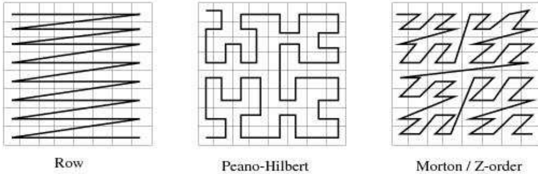
Figure 10: Space-filling curves to linearize a multidimensional space
