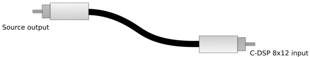
Figure 1. Single-ended RCA connection
