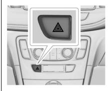
$\triangle$ : Press and momentarily hold to make the front and rear turn signal lamps flash on and off. This warns others that you are having trouble. Press and momentarily hold again to turn the flashers off.
