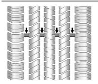
Treadwear indicators are one way to tell when it is time for new tires. Treadwear indicators appear when the tires have only 1.6 mm (1/16 in) or less of tread remaining. See *Tire Inspection*  $\Rightarrow$  232 and *Tire Rotation*  $\Rightarrow$  232.
