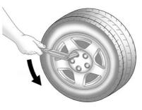
2. Turn the wheel wrench counterclockwise to loosen the wheel nuts. Do not remove them yet.
