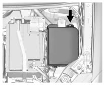
To remove the fuse block cover, squeeze the clip and lift it up.
