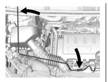
Lift the hood and release the hood prop rod from its retainer, in the front of the engine compartment. Securely insert the rod end into the slot marked with an arrow, on the underside of the hood.
