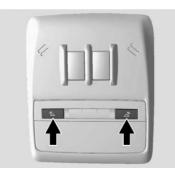
The front reading lamps are in the overhead console.
