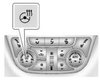
If equipped, press to turn on or off. A light on the button displays when the feature is turned on. The steering wheel takes about three minutes to start heating.
