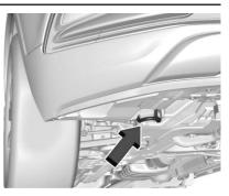
The vehicle is equipped with a specific attachment point to be used by the towing provider. This point may be used to pull the vehicle from a flat road surface onto the flatbed tow truck.
