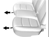
Pull the strap on the front edge of the rear seat cushion to release the cushion. Tilt the seat cushion forward toward the front of the vehicle.
