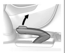
To set the parking brake, hold the brake pedal down and pull up on the parking brake lever. If the ignition is on, the brake system warning light will come on. See *Brake System Warning Light*  $\Rightarrow$  105.
