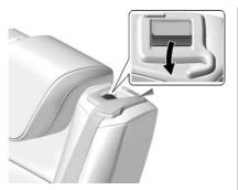
6. Reach under the belt and pull the lever on top of the seatback to unlock the seatback.
