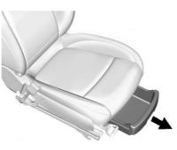
If equipped, there is storage under the front passenger seat. Lift the end of the tray and pull it forward to open. Push it in toward the seat to close.
