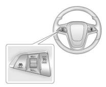
\*\*\*\*\* : Press to turn the cruise control system on or off. A white indicator comes in the instrument cluster when cruise is turned on.
