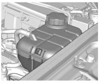
Check to see if coolant is visible in the coolant surge tank. If the coolant inside the coolant surge tank is boiling, do not do anything else until it cools down. If coolant is visible but the coolant level is not at or above the mark pointed to, add a 50/50 mixture of clean drinkable water and DEX-COOL coolant.
