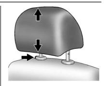
The height of the head restraint can be adjusted. Pull the head restraint up to raise it. Try to move the head restraint to make sure that it is locked in place.
