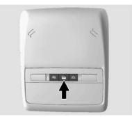
The front dome lamp controls are in the overhead console.
