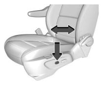
If available, press the front or rear of the switch to increase or decrease lumbar support. Release the switch when the desired level of support is reached.
