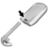
1. Press the button on the back of the RKE transmitter and pull the key out. Never pull the key out without pressing the button.
