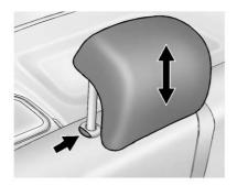
To lower the head restraint, press the button, located on the top of the seatback, and push the head restraint down. When an occupant is in the seat, always return the head restraint to the upright position. Pull the head restraint up and push it rearward until it locks into place. Push and pull on the head restraint to make sure that it is locked.
