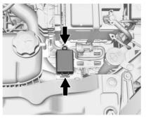
To remove the fuse block cover, squeeze the clips and lift it up.
