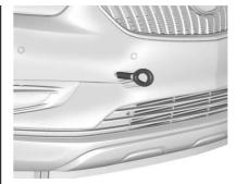
Install the tow eye into the socket by turning it clockwise until it stops. When the tow eye is removed, reinstall the cover with the notch in the original position.
