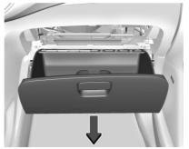
2. Push in both sides of the glove box and pull to remove.
