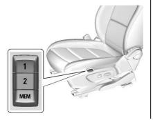
If equipped, the MEM, 1, and 2 buttons on the outboard side of the driver seat are used to manually save and recall the driver seat and outside mirror positions. These manually stored positions are referred to as Button Memory positions.
