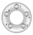
13. Tighten the wheel nuts firmly with the wheel wrench in a crisscross sequence, as shown.
