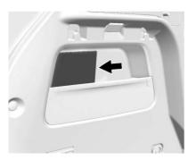
The rear compartment fuse block is behind a cover on the driver side of the rear compartment. To access the fuses, remove the cover.
