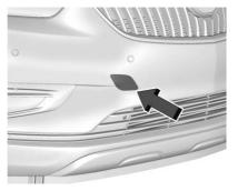
If equipped, carefully open the cover by using the small notch that conceals the tow eye socket.
