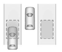
The SBZA sensor covers a zone of approximately one lane over from both sides of the vehicle, or 3.5 m (11 ft). The height of the zone is approximately between 0.5 m (1.5 ft) and 2 m (6 ft) off the ground. This zone starts at approximately the middle of the vehicle and goes back 5 m (16 ft).
