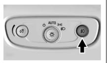
The fog lamps button is on the instrument panel beside the steering wheel.
