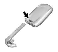
To remove the key, press the button on the back of the transmitter, and pull the key out. Never pull the key out without pressing the button.
