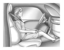
If a person of adult size is sitting in the front outboard passenger seat, but the OFF indicator is lit, it could be because that person is not sitting properly in the seat. Use the following steps to allow the system to detect that person and enable the front outboard passenger frontal airbag and knee airbag (if equipped):
