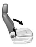
3. Lift the lever fully and fold the seatback forward.
