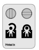
If equipped, the safety lock is located on the inside edge of the rear doors. To use the safety lock:
