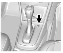
4. Insert and push the key into the slot.
