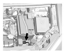
2. Open the hood and unwrap the electrical cord. The cord is in the driver side of the engine compartment, near the battery. It is shipped from the factory with a tie holding it in place. Use care in removing the tie so that the cord is not damaged.
