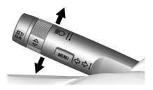
ED : Push the turn signal lever away from you and release, to turn the high beams on.
