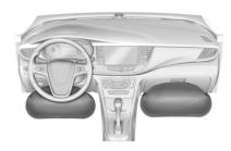
The driver knee airbag (if equipped) is below the steering column. The front outboard passenger knee airbag (if equipped) is below the glove box.
