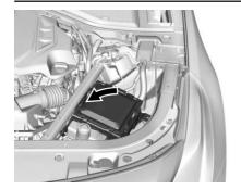
Lift the fuse block cover to access the fuses.
