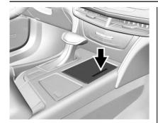
There are cupholders in the center console. Push and release on the passenger side of the cover to access the cupholders.
