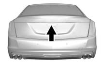
Press the touch pad on the rear of the trunk above the license plate when all doors are unlocked. For Keyless Access, the trunk can be opened while the vehicle is locked by pressing the touch pad above the license plate while the RKE transmitter is within 1 m (3 ft) of the rear of the vehicle. See *Remote Keyless Entry (RKE) System Operation*
