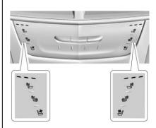
If equipped, the buttons are near the climate controls on the center stack. To operate, the ignition must be on.
