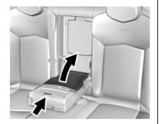
Press the latch to access the storage area in the rear armrest. Press the button to extend the cupholders.
