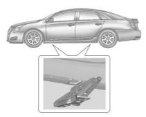
Position the jack lift head at the jack location nearest the flat tire within the depression of the jack pads, as shown. The jack must not be used in any other position.
