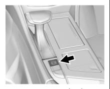
Automatic Vehicle Hold (AVH), if equipped, can be turned on by pressing AUTO HOLD with the driver seat belt fastened, the driver door closed, and the engine running. The AVH indicator will come on.
