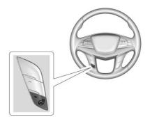
**3**: If equipped with a heated steering wheel, press to turn on or off. An indicator next to the button is lit when the feature is turned on.
