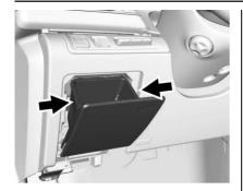
Apply pressure to the two retaining tabs on the sides of the compartment, until the two retaining tabs clear the sides of the instrument panel. Allow the compartment to move downward, and out of the way.
