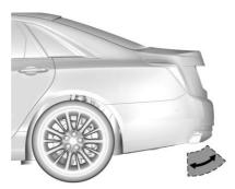
To operate, kick your foot straight up in one swift motion under the center of the rear bumper, then pull it back.
