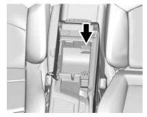
Place the new transmitter in the transmitter pocket. The center console storage area will need to be opened.
