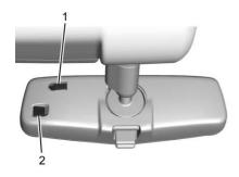
To adjust the brightness, press the button (1) on the back of the rearview mirror without covering the light sensor (2).
