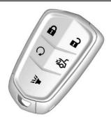
**a**: Press to lock all doors. The turn signal indicators may flash and/or the horn may sound on the second press to indicate locking. See *Vehicle Personalization*
