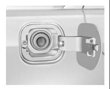
To open the fuel door, push and release the rearward center edge of the door. If equipped, the fuel door is locked when the vehicle doors are locked. Press a on the RKE transmitter to unlock.
