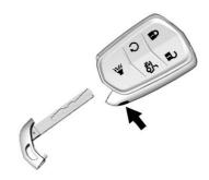
Press the button to remove the key. The key can be used for the driver door.
