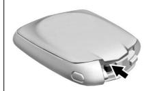
Separate the two halves of the transmitter using a flat tool inserted into the bottom center of the transmitter. Do not use the key slot.
