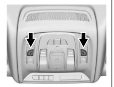
Press ₩ or ₩ next to each overhead console reading lamp.
