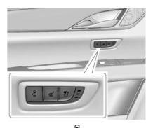
If equipped, press a to tilt the front of the seat fully downward and to move the entire seat fully rearward. The seat will also move to this position when the rear door is opened.
