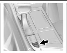
Press and release MODE to activate the mode menu in the instrument cluster. The first press of the button will show the current mode.
