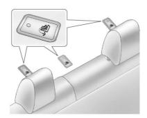
The top tether anchors are behind the rear seat, on the filler panel. Open the covers to access the anchors. Be sure to use an anchor on the same side of the vehicle as the seating position where the child restraint will be placed.
