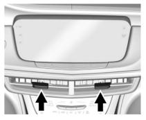
Adjustable air vents are in the center and on the sides of the instrument panel, on the rear of the center console storage, and in the headliner over the rear seats, if equipped.
