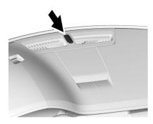
The vehicle has a Charging Status Indicator (CSI) at the center of the instrument panel near the windshield. When the vehicle is plugged in and the vehicle power is off, the CSI indicates the following:
