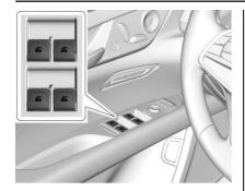
Power windows work when the ignition is on, in ACC/ACCESSORY, or when Retained Accessory Power (RAP) is active. See *Retained Accessory Power (RAP)* ⇒ 227.
