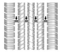
Treadwear indicators are one way to tell when it is time for new tires. Treadwear indicators appear when the tires have only 1.6 mm (1/16 in) or less of tread remaining. See *Tire Inspection*  $\Rightarrow$  375 and *Tire Rotation*  $\Rightarrow$  376.
