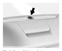
The indicator light, on the instrument panel near the windshield, indicates the status of the system. On the PLUG-IN, the Charging Status Indicator is integrated into the indicator light. See *Charging Status Feedback (PLUG-IN Only)* ⇒ 294.
