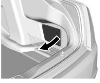
The rear compartment fuse block is behind a cover on the passenger side of the rear compartment.
