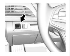
The vehicle has an Electric Parking Brake (EPB). The EPB can always be activated, even if the ignition is off. To prevent draining the battery, avoid repeated cycles of the EPB system when the engine is not running.
