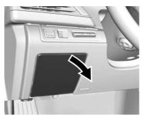
The storage compartment has a press to open latch. To access the fuses, open the compartment by pressing and releasing near the top center square.
