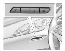
If equipped, memory seats allow two drivers to store and recall their unique seat positions for driving the vehicle, and a shared exit position for getting out of the vehicle. Other feature positions may also be set, such as power mirrors and power steering wheel. Memory positions are linked to RKE transmitter 1 or 2 for automatic memory recalls.
