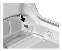
Insert an SD card into the card reader in the trunk. Disable recording from the playback screen before removing the SD card from the reader. Do not remove the card while recording is enabled. This could corrupt the video file and/or the SD card.
