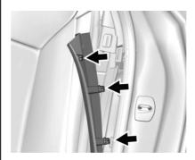
Remove the trim molding by pulling until the top three attachments are removed.
