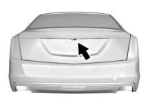
The camera that provides the Rear Camera Mirror (RCM) image is above the license plate, next to the Rear Vision Camera (RVC).
