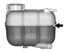
The coolant surge tank is in the engine compartment on the passenger side of the vehicle. See Engine Compartment Overview \$ 320.
