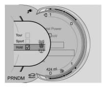
Use Hold Mode on a trip where it is expected that all of the electric charge will be depleted. Use Hold Mode mainly during highway or high speed driving to maximize both PLUG-IN propulsion miles and fuel efficiency.
