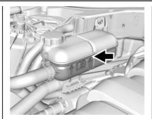
Check to see if coolant is visible in the reservoir. If coolant is visible but the coolant level is below the indicated mark, there could be a leak in the cooling system.
