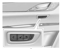
If equipped, press 🖥 to tilt the front of the seat fully downward and to move the entire seat fully rearward. The seat will also move to this position when the rear door is opened.
