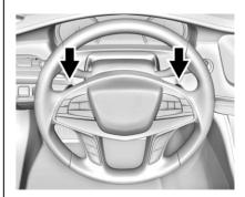
While using Regen on Demand, the vehicle will have increased coast deceleration. Use this to maximize regenerative braking, for sport driving, or when descending hills.
