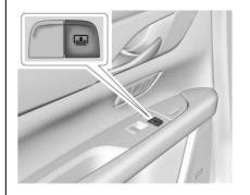
The rear door panels have controls for the rear sunroof sunshade. Press to open or close.
