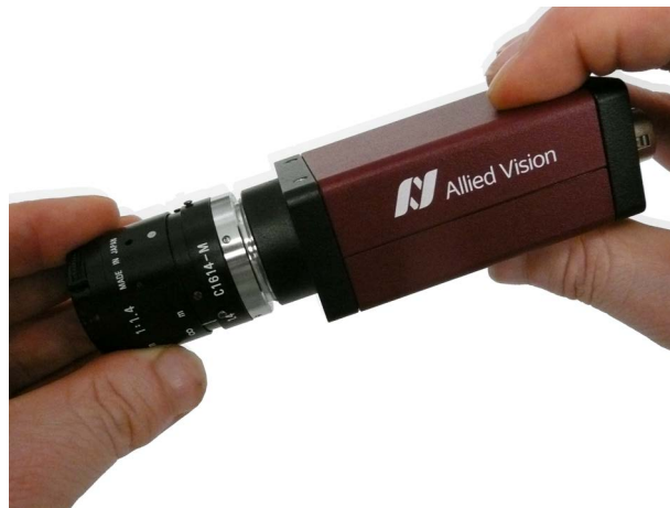
Figure 144: Illustration of camera orientation when removing lens or dust cap
