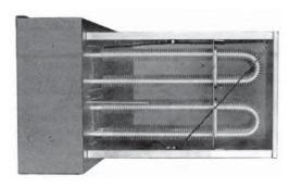
A manual secondary linear limit cutout protects against failure of the primary overtemperature system. With a fixed temperature setting higher than either of the primary cutouts described above, this device is designed to trip only if both of the primary cutouts stick in the closed position, or controlling contactor points weld together.
