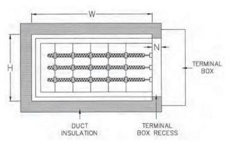
Figure 66. Installation of slip-in heater where insulation is more than 1" (25.4 mm) thick
