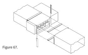
This option for custom flanged heaters, allowing installation with conventional HVAC slip-and-drive connections, offers the rugged and secure mounting of a flanged heater, yet requires less installation labor than a slip-in heater. It is particularly useful when other equipment in the duct system uses slip-and-drive connections, as the contractor can standardize throughout (Figure 67).
