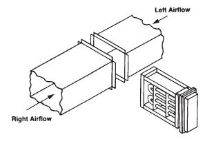
Figure 87. Standard Flanged Heater Installation
