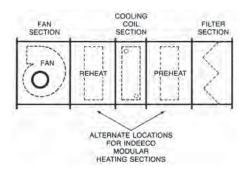
Multi-Zone or Dual Duct Heaters – These heaters are designed for installation inside multi-zone or dual duct air conditioning equipment, where the airflow is highly variable and unevenly distributed (Figure 51). These heaters use coils derated to approximately 25 watts per square inch (3.8 watts per square cm) of wire surface area (approximately one half normal watt density). Low density coils run cooler, and thus, provide longer life under these stringent operating conditions.
