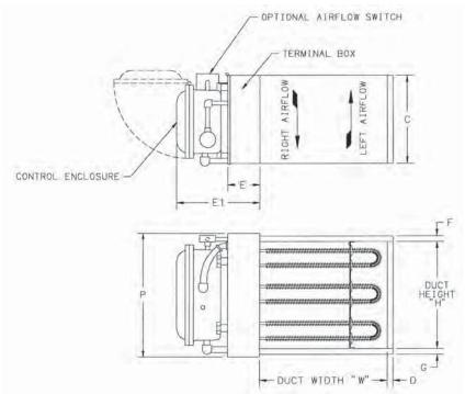
Figure 84. Dimensional Drawing for EP2
