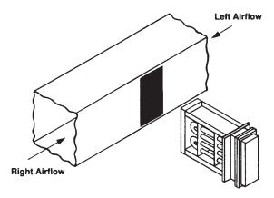
Figure 88. Optional Slip-in Heater Installation
