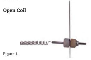
Only the highest Grade A resistance wire (80% nickel, 20% chromium) is used in all Indeeco duct heaters. This iron-free wire has a higher maximum operating temperature, greater life, lower sag, less resistance change and higher corrosion resistance than other commonly used resistance wires.
