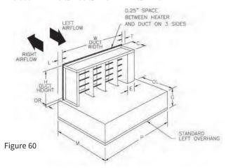
The NEC requires a work space at least 30" (76 cm) wide by 42" (107 cm) deep in front of a heater terminal box for service access. More space is required for large heaters. When this space is not available at the side of a duct, the heater can be installed through the bottom, using a special bottom mounted terminal box construction, which maintains the required horizontal orientation of open coil resistance elements.
