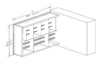
Figure 69. Slip-in Duct Heater
