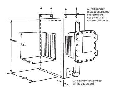
Maximum duct dimensions (W<sub>Max</sub> & H<sub>Max</sub>) should allow for 1" minimum flange all around.
