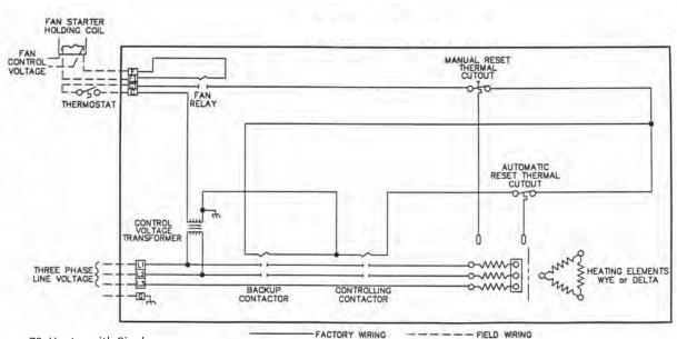
Figure 79. Heater with Single Stage Control
