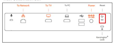
The following figure shows the reset key located on the base of the C470HD.
