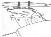
Fig. 317 righthand plenum panel cover retaining screw locations. 1998-2005 Volkswagen New Beetle
