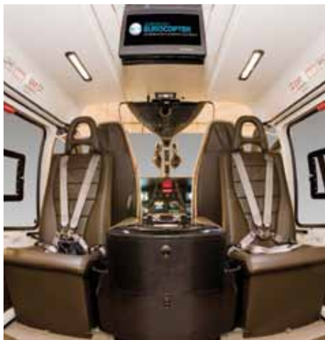
LCDs from Flight Display Systems are mounted from the ceiling of this EC145.
