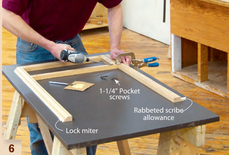
6 Assemble the face frame with glue and pocket screws. Clamp the frame to a flat surface to ensure good alignment, taking care not to damage the lock miter.
