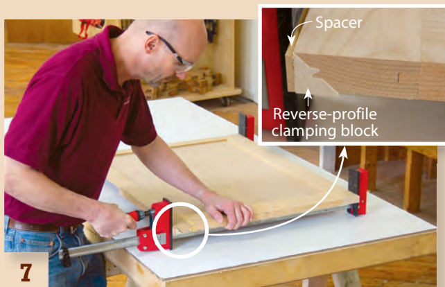
7 Glue together the side panel. Protect its delicate lock-mitered edge by using a spacer and shop-made clamping blocks with the reverse profile.
