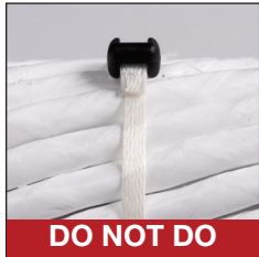
Fig. 22 Cut end of lacing tape is too short
