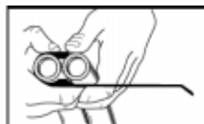
2. Position second hose in clamp.
