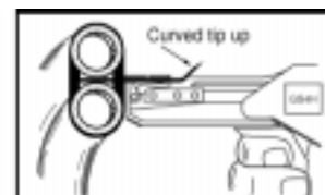
4. Tension and cut off with Panduit tool.
