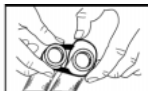
3. Loop tail around second hose and thread tail through both spacer heads.
