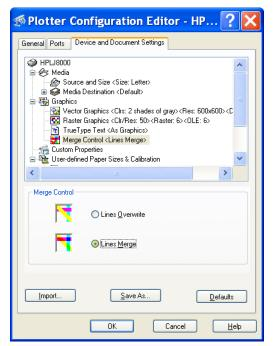
Select the Device and Document Settings tab and then select the plus symbol to the left of the 'Graphics' option. This will display the options, select the 'Lines Merge' option as shown in **Figure IV -26.**
