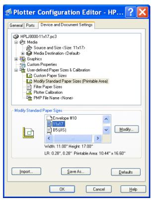
Next, select Ok to exit the Plotter Configuration Editor as shown in Figure IV -31.
