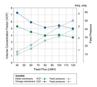
The range of operating VCF can be determined for a specific feed solution by doing a feed flux excursion.
