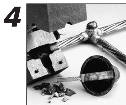
Open the mold and remove the expended steel cup – no special disposal required
