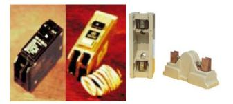
The current ratings of fuses and circuit breakers are so high (15 to 30 amperes for most residences) that they cannot protect against shock. When the current flow exceeds the rated levels, the fuse melts or the circuit breaker is tripped. In either case, the circuit is broken and current can no longer flow.
