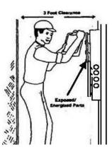
Wall not grounded. e.g. Plasterboard on Wood Studs
