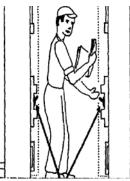
Motor control centers with live parts at relays and conductors exposed
