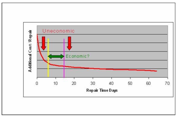
Figure 3. Additional cost of repair with reduced repair time
