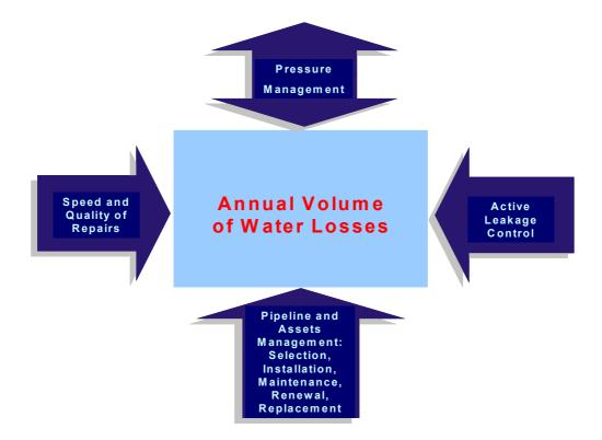
Figure 1. The four primary components of leakage management
