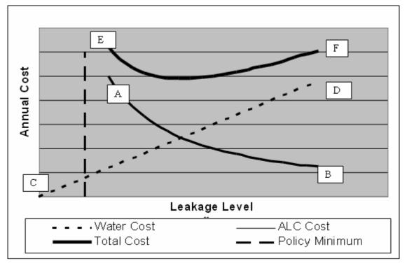
Figure 2. Active Leakage Control (ALC) cost curve
