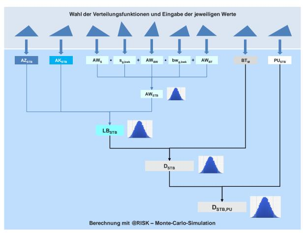
Figure 3: Calculation Mode 3 – construction time: Flow chart
