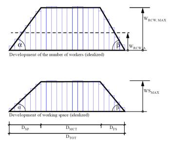
Figure 2: Correlation between number of workers and available workspace for reinforced concrete works
