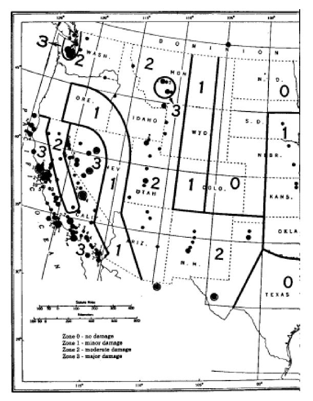
Figure 4 1952 UBC Seismic Zones in Washington State (Washington State Zones do not change for 1955, 1958, 1961 and 1964 UBC)
