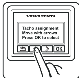
13. Allocate tachometer. Scroll using the arrow buttons.
