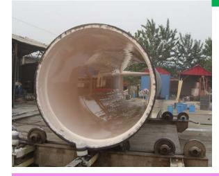
Polyethylene lining pipes
